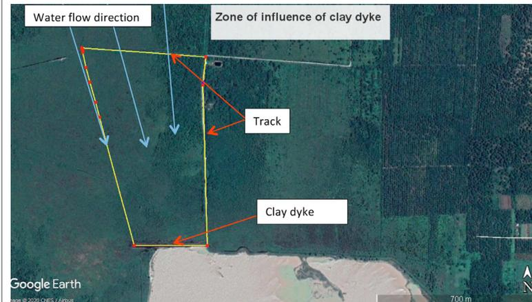
Figure 7. The direction of water flow across the landscape and the resulting 'zone of influence' of the clay dyke (shown by the yellow outline). Figure and associated area calculations were provided by the project contact.
