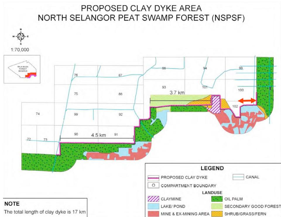
Figure 2. The proposed total length of clay dyke to be constructed between the ex-mining area and the Raja Musa Forest Reserve (the project dyke section is shown with a red arrow).
