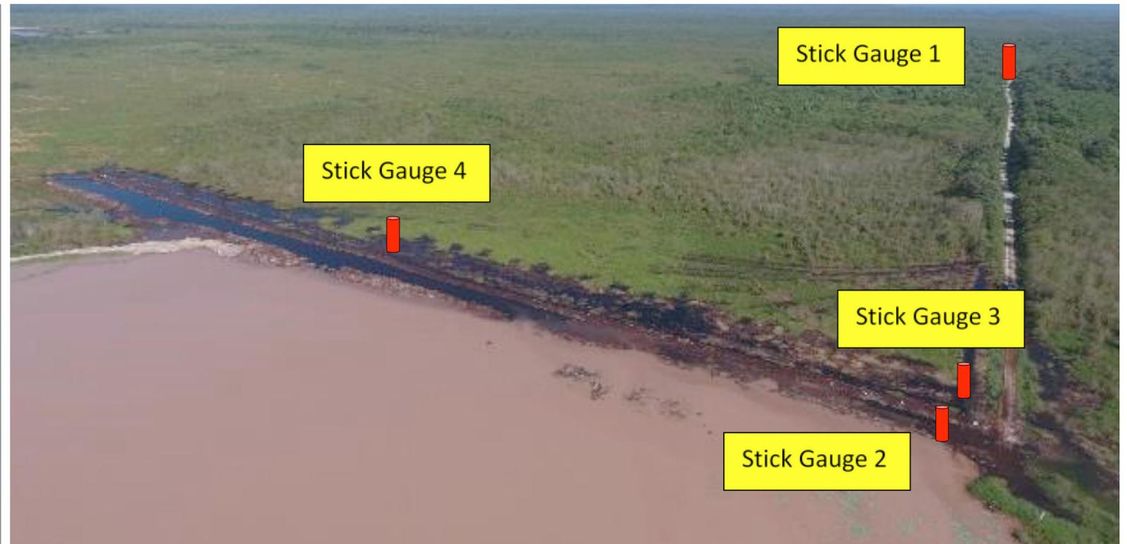
Figure 6. Location of stick gauges installed along and behind the clay dyke. The peatland is the area with higher levels of vegetation, in the background of the photo. The water body in the bottom of the photo is the area marked "lake" in Figure 5.
