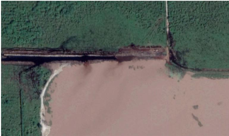
Figure 11. Aerial photo in the same location as Figure 8, taken January 1<sup>st</sup>, 2020. This image shows the nearly completed clay dyke as well as the high water level in lake. Note that the water (estimated to be about 1.5m higher than in August 2017) is covering the lake shore and sand spit.
