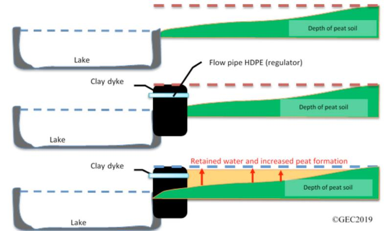
Figure 5. Clay dyke design, showing the previously existing water body (top), the area directly after construction (middle), and the intended water retention (bottom).
